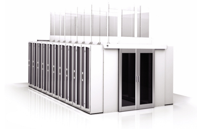
Figure 6: Standard Hot Aisle Containment Solution by CPI. In the example above, CPI's Aisle Containment Doors are combined with the F-Series TeraFrame® Cabinet System and an overhead duct to enclose the hot aisle between adjacent cabinet rows and the overhead duct is used to isolate hot exhaust air from the room.
