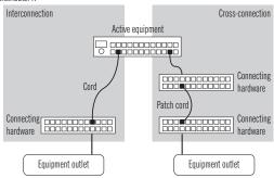
Figure 15 – Interconnections and cross-connections
