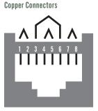
Figure 9a – IEC 60603-7 series interface for Category 5, 6 and 6A. Please note the categories refer to the IEC requirements and not the TIA-568 range of standards.
