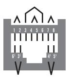
Figure 9b – IEC 60603-7 series interface for Category 7 and 7A. Please note the categories refer to the IEC requirements and not the ANSI/TIA-568 range of standards.
