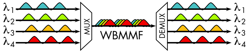
Figure 5 - WDM concept showing four wavelengths
